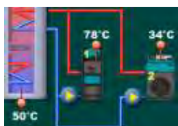
Tank reheating: example 1 wood boiler and 1 oil/gas boiler - control unit controls only the boiler pumps, do not switch off/on the boilers!
