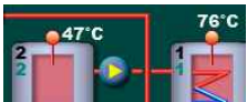
Mixing / reheating Reheating – Pump between the accumulation tank and DHW tank for reheating of the DHW tank
