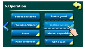
This option is used to set pellet delivery vacuum suction system.
