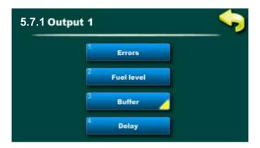
\* By pressing this button user can disable/enable the fuel level warning sound from the speaker. (It refers only to warning about the low fuel level in the tank when speaker is selected as connected device). If only lamp is connected and selected as connected device, this shortcut is not displayed.
