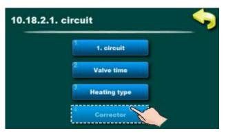
Enable the corrector in the heating circuit
