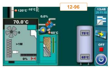
When "1 Temperature" is selected, screen shows hydraulic crossover with 1 temperature (not possible at 69/96).
