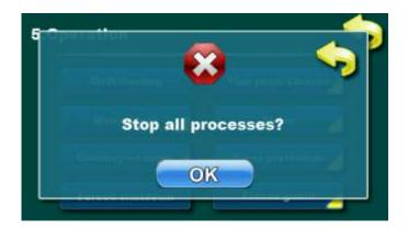
IMPORTANT! To be able to stop all processes, you must first turn off the boiler in the usual way by pressing on and then STOP.
