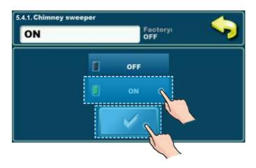
When this option is turned ON, button "BOILER OPERATION DISPLAY" becomes a button "CHIMNEY SWEEPER" (1). Pressing this button directly opens the menu "CHIMNEY SWEEPER" (without the need for scrolling through the menus). In this menu, is access to change parameters of "CHIMNEY SWEEPER" menu.
