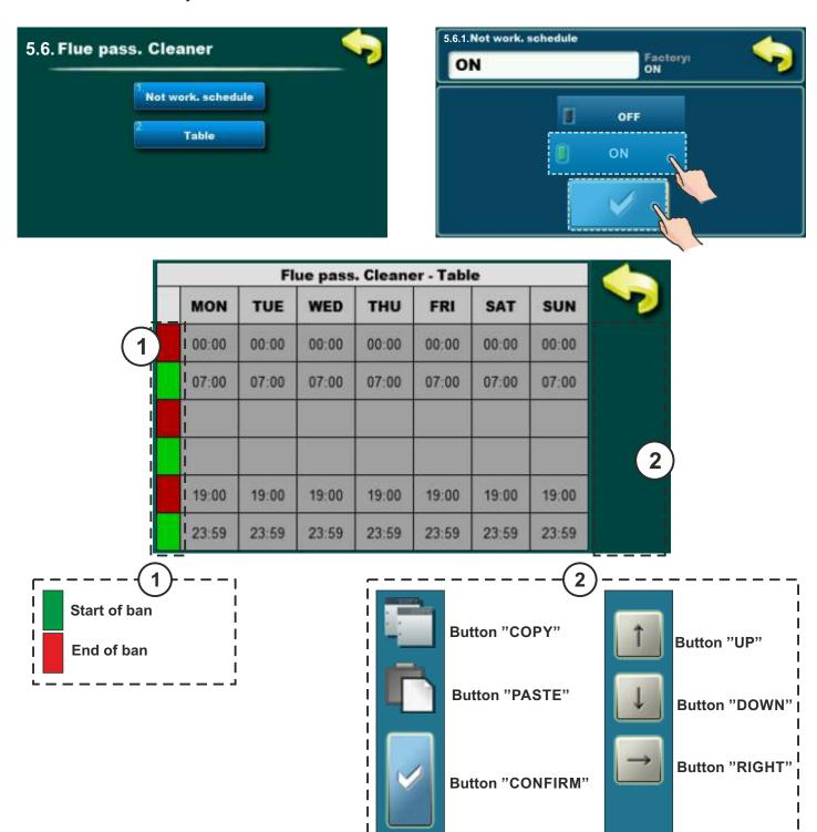
According to the data in the table, cleaning the flue passage is banned from 0:00 to 7:00 and from 19:00 to 21:00 every day of the week. This means that boiler will clean the flue passages only during the period from 07:01 to 18:59. Table can be adjusted according to the needs in the same way as the table "Schedule" (see 3.2-3.4).
