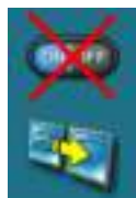
All elements of automatic / remote boiler start are disabled (ON/OFF button is crossed in red)
