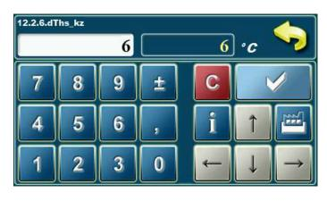
Factory settings: 6°C Possible selection: min. 1°C, max. 15°C a) for connection method CRO (Hydraulic crossover)
