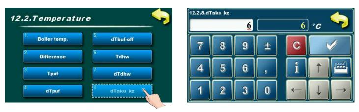
Factory settings: 6°C Possible selection: min. 1°C, max. 15°C a) for connection method CRO + sensor (Hydraulic crossover + sensor)
