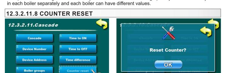
This parameter enable reset of boiler work time counter. It can be reset on each boiler separately.
