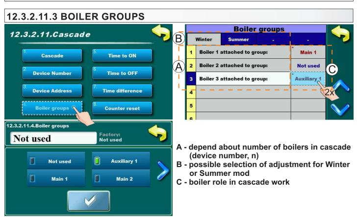
By pressing on menu "C" on display will be opened menu for choice boiler role in cascade work. Boiler role is adjusted for Winter and Summer work mode seperately (menu "B").
