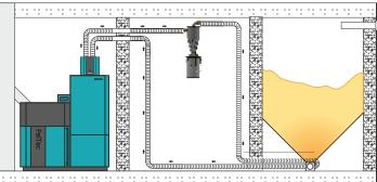
The cyclone is used for dust extraction from pellet suction feeding system in order to prevent dust accumulation in seasonal pellet storage through a longer usage period - LEFT.
