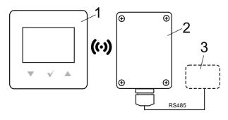
Radio communication: 1 – HPx40CM thermostat, 2 – HPrfCM radio module, 3 – HPCU360iCM control unit.
