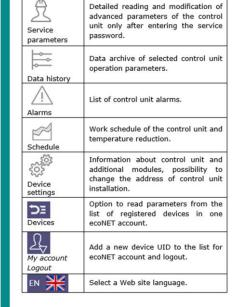
The **Current Data** tab includes tiles with values of basic control unit operation parameters. A parameter to be modified is
