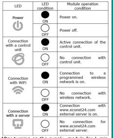
After turning on the supply, module for 1 min it loads the system, only after this time it starts working.
