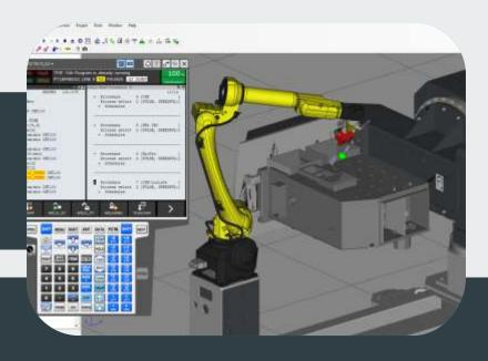
Robotic welding is an automated process that uses industrial robots to perform welding operations. This technologically advanced approach enables high precision, consistency and efficiency in welding metal components. MAG pulse welding and Servo-Robot laser cameras are used for reading, which enable repeat accuracy during welding.
