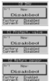
Configuration: boiler + accumulation tank + protection valve + return flow sensor + DHW
