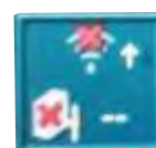
Regulation is not connected with web portal (internet supervision is not possible)
