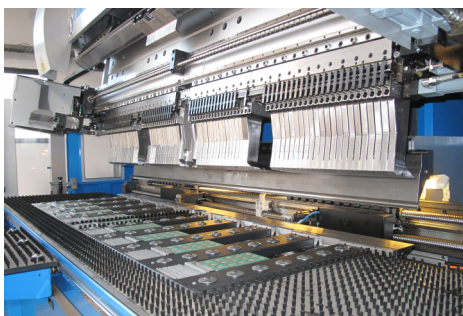
Bending and perforation of metal sheet with modern CNC machines
