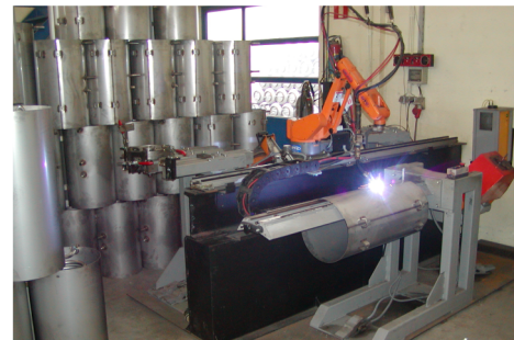
Robotic welding of stainless steel water heaters
