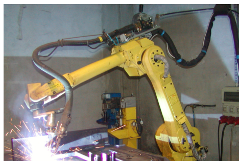
Robotic welding of the boilers
