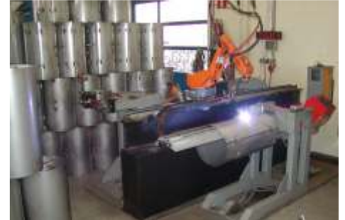
Robotic welding of stainless steel water heaters
