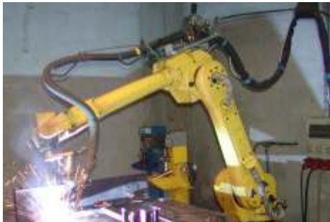
Robotic welding of the boilers
