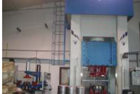
Forming of metal sheet with hydraulic presses
