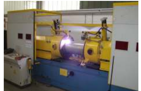
Automated welding of stainless steel water heaters
