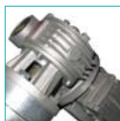
Motor reducer of the pellet conveyor
