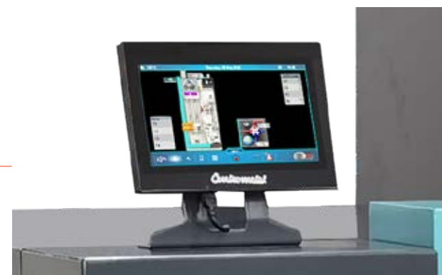
Multifunctional digital controller with a 7" touch screen
