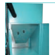
Pellet tank cleaning openings
